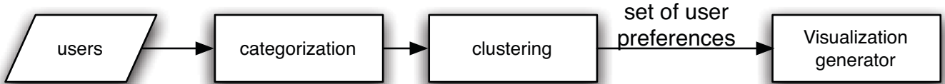
Figure 2. Our approach consists of four steps: 1) categorized the user depending on device used. 2) group users according to profiles similarity 3) set the user preferences 4) use these preferences to generate a customized visualization
