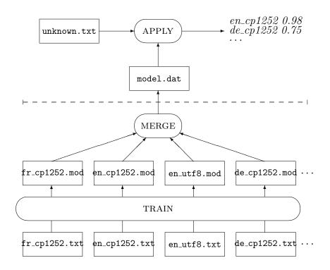
Figure 2: SILC system architecture. Individual model files \*.mod are generated by train from text files \*.txt, then combined into a single grouped model file model.dat by merge. This file is then used by apply to determine the language and encoding (here English and cp1252) of the content of unknown.txt.
